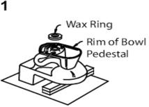
Clean the immediate floor area thoroughly. Insert new toilet bolts in the slotted flange, bolt heads down. The toilet should be placed on the floor upside down, on soft material to prevent scratching. Place the slightly warmed wax ring in the circular recess in the base of the bowl.
