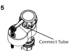
Connect the plastic tubing from the top of the water inlet regulator into its holding ring inside the overflow tube. If necessary, excess may be trimmed to eliminate any leaks.
