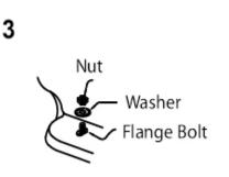
Place the washers (Marked: This Side Up) and nuts on the bolts. Alternately finger tighten then 1/2 turn with a wrench. DO NOT OVERTIGHTEN NUTS AS CHINA EASILY CHIPS AND CRACKS. Pour water into bowl to prevent the escape of sewer gas. Trim bolt height if required, to place caps. Wipe away any excess sealant at pedestal base along floor line.
