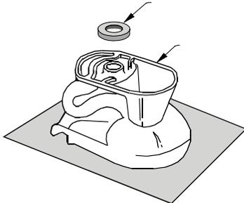
Clean the immediate floor area thoroughly. Insert new toilet bolts in the slotted flange, bolt heads down. The toilet bowl should be placed upside down, on soft material to prevent scratching. Place the slightly warmed wax ring in the circular recess in the base of the bowl.
