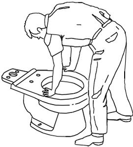
Unplug floor waste opening. Gently place the bowl, right side up, in position with the toilet mounting bolts protruding through the holes in the china base. Press down, with a slight twisting motion, on the top center, with your full weight. Make sure the bowl is as level as possible. If needed, you can use wedges under the bowl to help leveling. Put the washers (Marked: This Side Up) and nuts on the bolts. Tighten them evenly and snugly.
