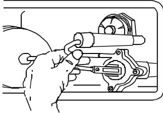
Connect the plastic tubing from the top of the water inlet regulator into its holding ring inside the overflow tube. If necessary, excess may be trimmed to eliminate any kinking of the line.
