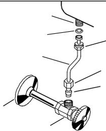
Connect the cold water line to the tank with your straight or angle stop. Place the washer, then the plastic nut on the tank end of the connecting pipe and bend the pipe to fit into the inlet hole on the water regulator. Tighten all coupling nuts securely. **DO NOT USE PLUMBERS PUTTY!**
