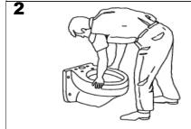
Place the felt or neoprene gasket on the bowl outlet. (wax ring is not recommended) When the bowl is installed, The gasket must be compressed sufficiently against the hub to effect a gas and watertight seal. NOTE: Bearing nuts and washers must be set to take full loading from the fixture allowing 1/16" clearance between fixture and wall. Follow support manufacturer 's recommended setting of closet outlet connection.
