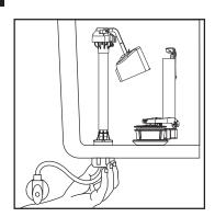
With correct washers in place (see Step 9a), tighten COUPLING NUT 1/4 turn beyond hand tight. DO NOT OVERTIGHTEN.
