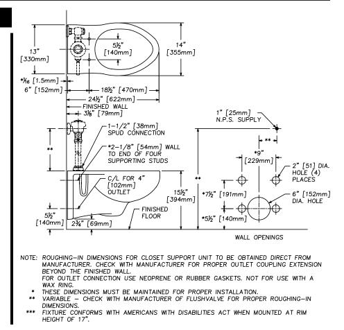
*IMPORTANT: These dimensions are nominal and may vary within the range of tolerances established by ASME Standard A 112.19.2 Contact your local building code for approved barrier free measurements.*
