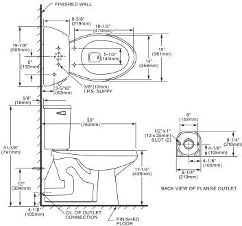
WASTE OUTLET SEAL RING MUST BE NEOPRENE OR GRAPHITE-FELT (WAX RING NOT RECOMMENDED). SUPPLY NOT INCLUDED WITH FIXTURE AND MUST BE ORDERED SEPARATELY.
